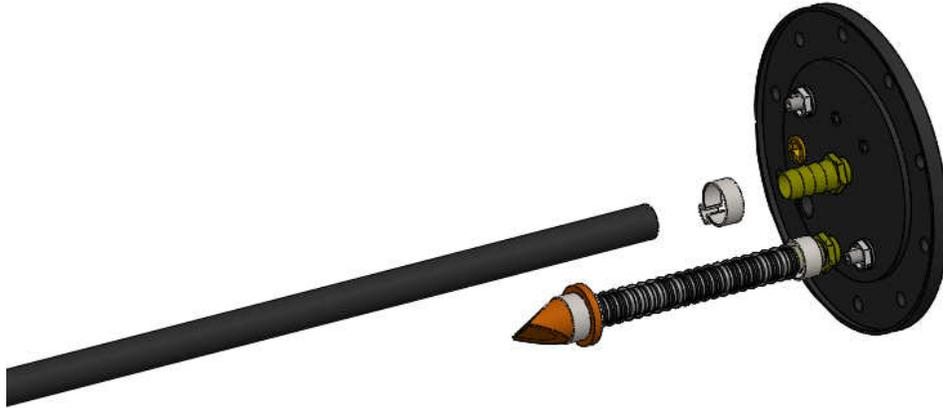
8. Using the 5/32" Allen wrench, install the longer fuel pump bracket from the extension kit. If you have lost any of the original hardware, don't worry, replacement hardware is included in your extension kit.
