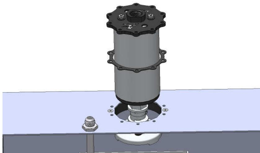
10. With the pump inserted into the tank, take the supplied socket head cap screws and washers and tighten them down. Do not over tighten as it will break or damage the washers. The finished product should look like **figure 1-8**.
