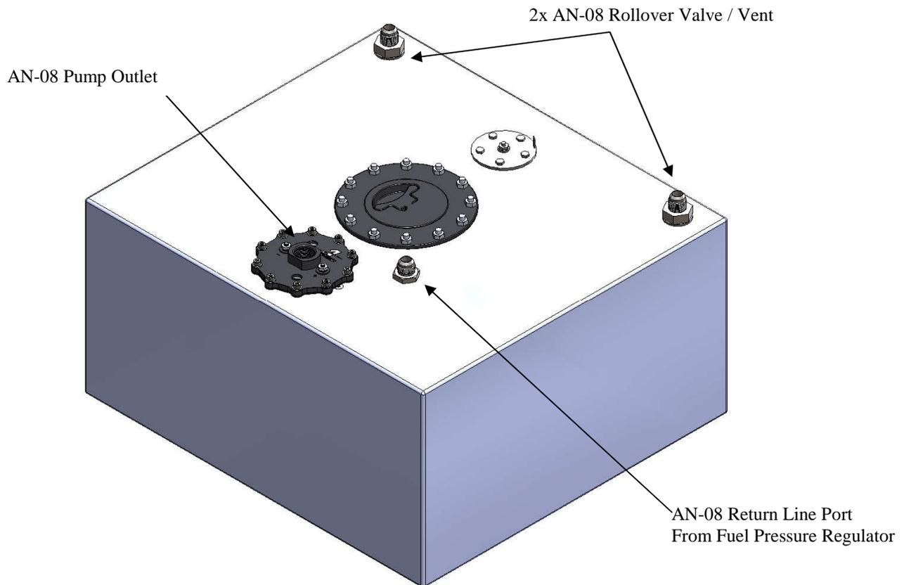
2. Connect AN-08 lines to the tank vent fittings. Tank vent lines must be ran outside the vehicle.
