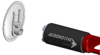
Position the fuel pump on the fuel pump hanger assembly such that from the bottom of the outlet cap to the bottom of the fuel pump strainer is equal to the fuel tank depth. Mark the bracket and the black outlet hose so they may be cut to the necessary lengths. Remember, take the time to measure twice and cut once!
