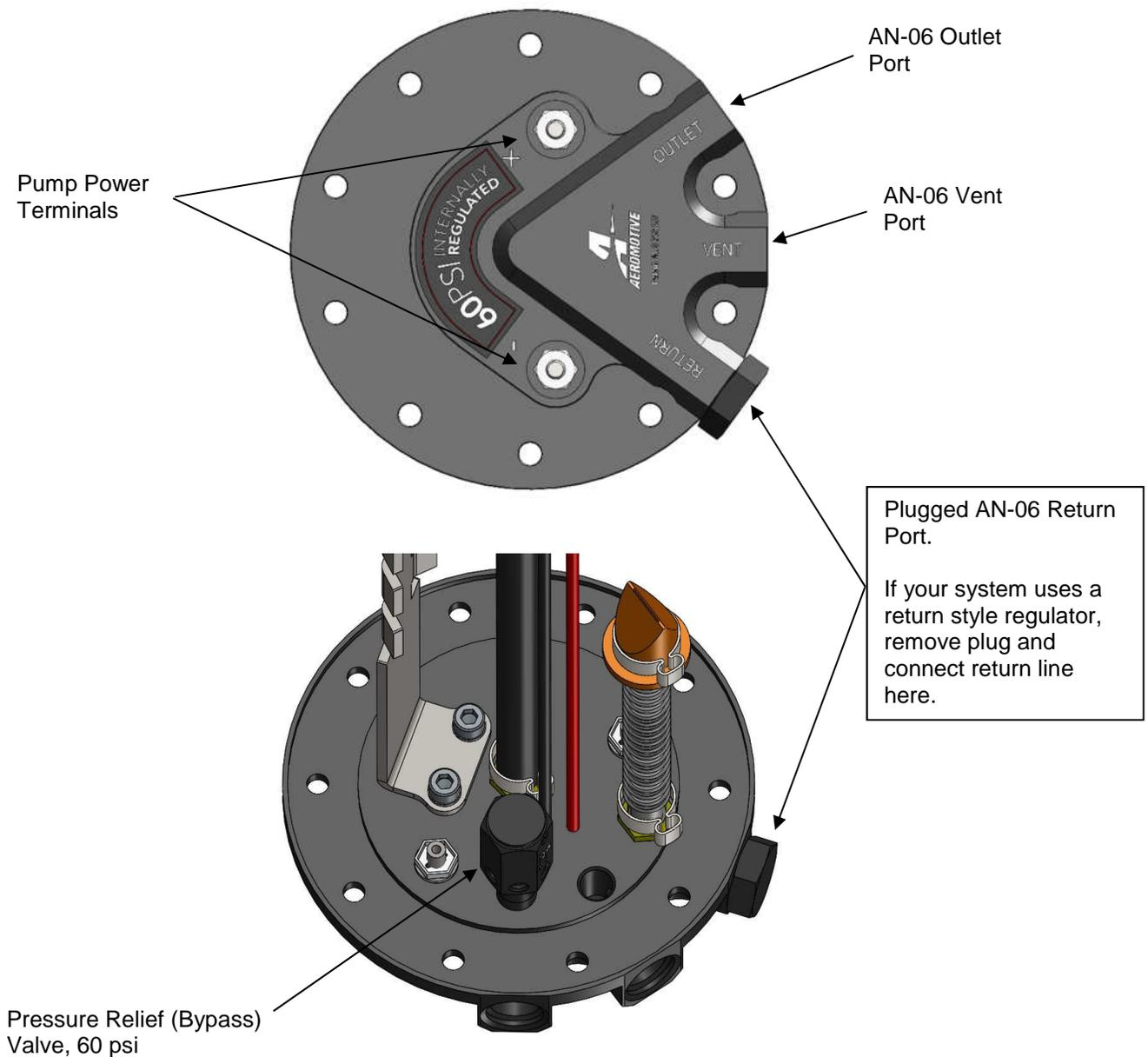
The enclosed Aeromotive fuel pump assembly utilizes an o-ring sealed AN-06 style feed, return (shipped with plug installed) and vent ports. These ports seal with o-rings; these ports are **NOT PIPE THREAD** and utilize **NO THREAD SEALANT**.
