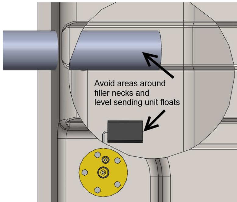
5. Secondly, locate and avoid areas of the top of the fuel tank that might contact the bottom of the vehicle frame rails, supports or floor pan.
