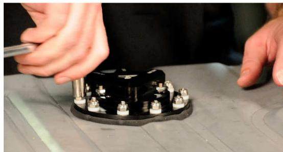
38. Prep the new tank by making all the necessary connections (feed, return, vent, and electrical) before placing tank in vehicle. In most cases, once the tank is placed in the vehicle these connections will not be accessible. For electrical wiring refer to **Figure 2-1** on the last page.
