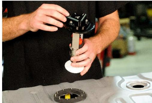
34. Press down firmly on the top of the pump assembly to compress the gasket. Start two of the 10-24 lock nuts on a pair of studs 180 degree apart. Tighten these two nuts until the remaining studs are approximately 1/4" exposed.
