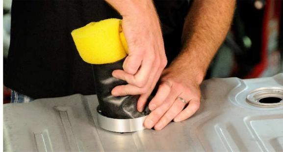
25. Install fuel pump strainer (pre-filter) on the fuel pump.
