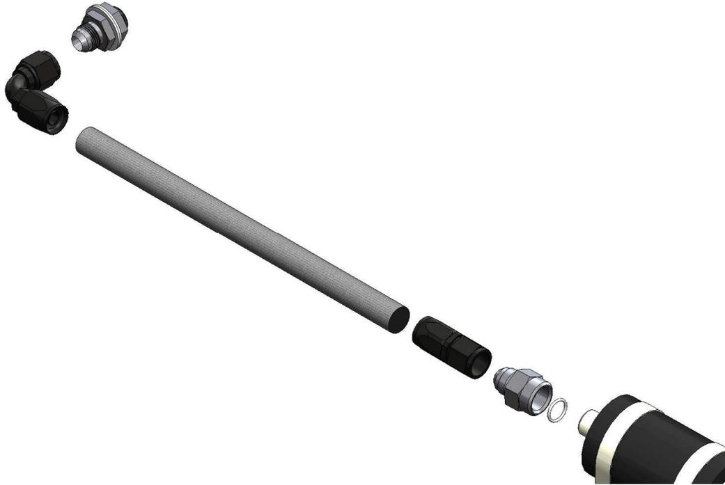
1-8. Install a short section of the 5/16" fuel injection rubber hose on the outlet side of the pump using one of the provided hose clamps.
