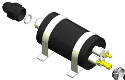
1-7. Plumb the inlet side of the prime pump using the supplied AN-08 hose and hose ends, refer to Section 2 for hose end installation instructions. It is recommended that a 100 micron fuel filter similar to Aeromotive 12316 be installed between the fuel cell and the primer pump.
