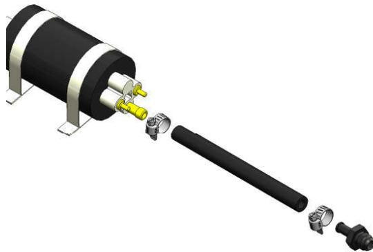
1-10. Install the AN-10 / AN-06 Port adapter fitting in the outlet of your fuel pump.
