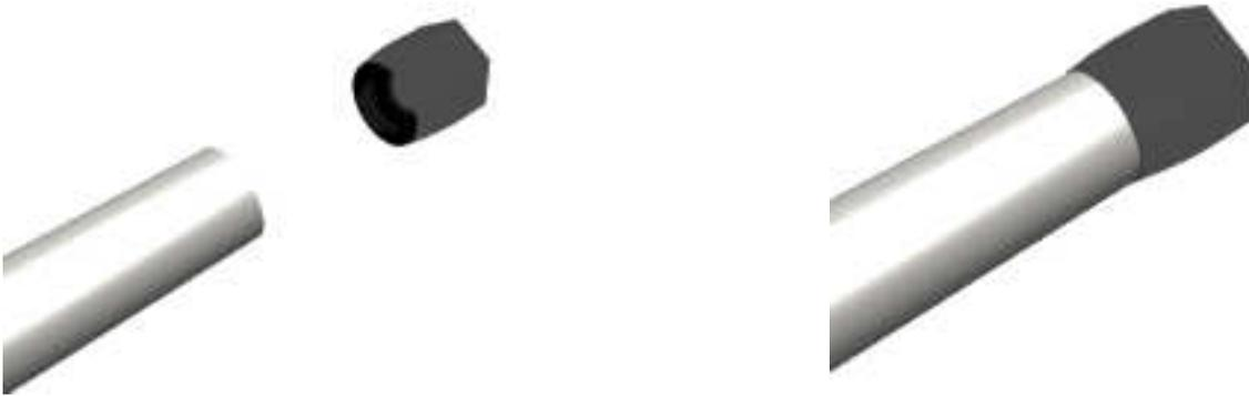
4-4. Using a grease pencil, marker or tape, mark the location of the hose in relation to the hose socket that you just installed.
