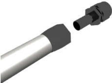
4-7. Using a properly sized wrench, complete threading the two components together (The maximum allowable gap between the two fitting components is .030 inches).
