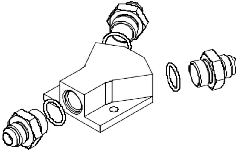
2-10. Starting from the fuel rails, plan a route to run an AN-08 supply line from each fuel rail to each side of the Y-block. Cut the two supply lines to the determined length and install the AN-08 hose ends, as detailed in Section 3.
