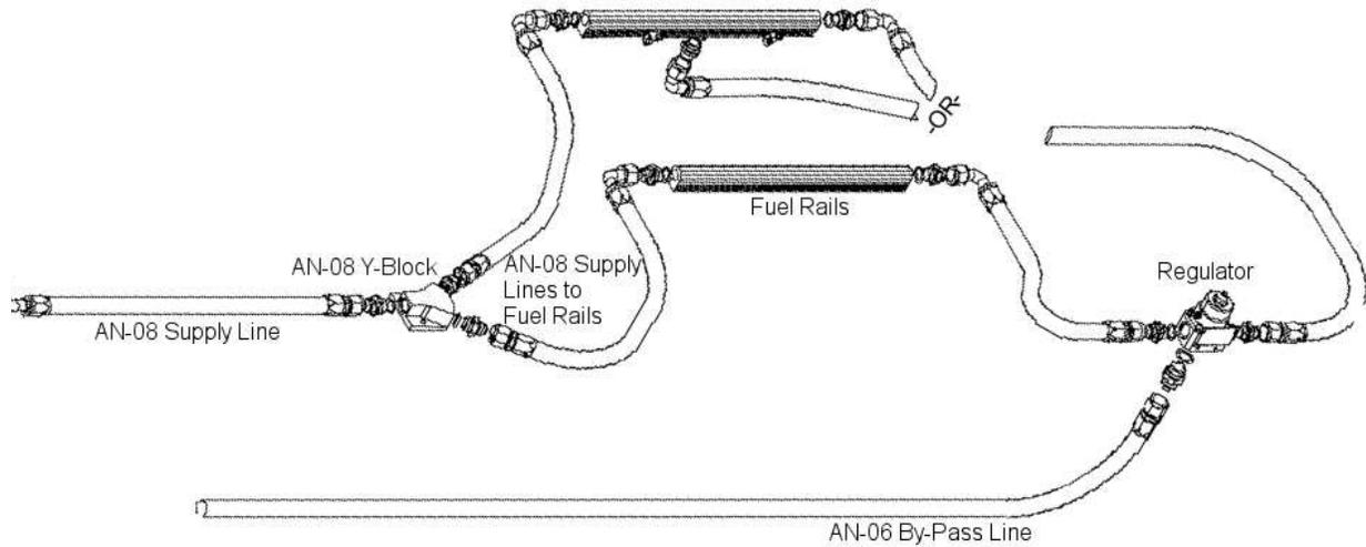
2-14. Once the regulator is installed, attach a suitable fuel pressure gauge (not supplied) to the 1/8 NPT port on the fuel pressure regulator.
