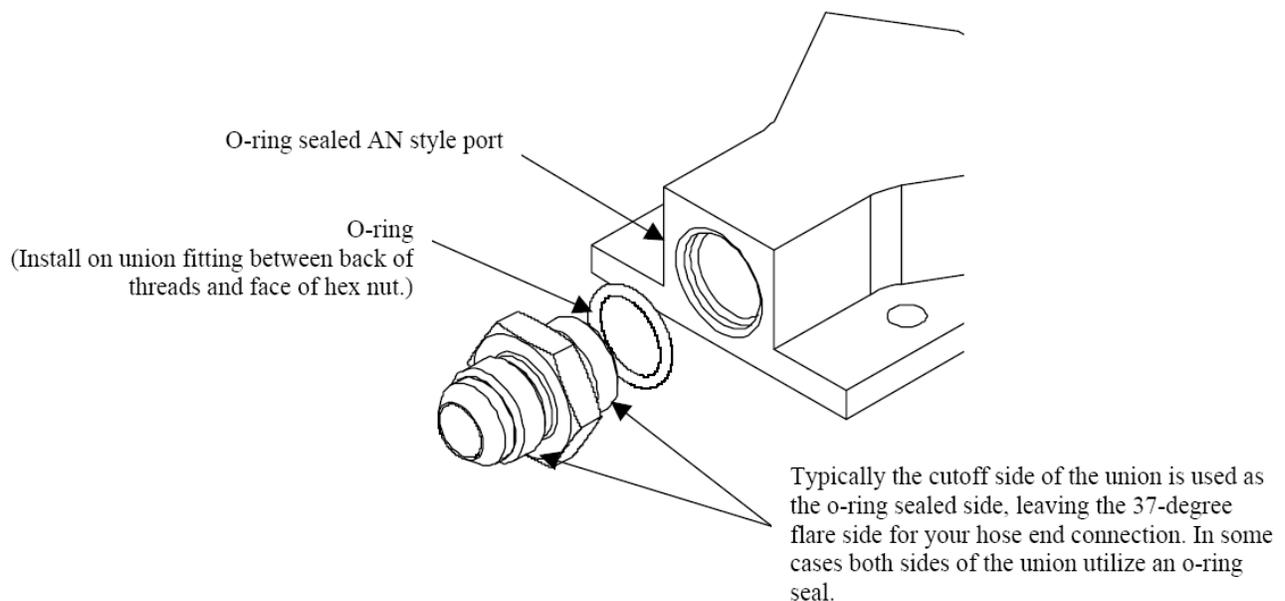
For example, in some systems an ORB to Flare fitting is used to connect the fuel pump and filter together, in which case you always install the ORB side into the fuel pump and the flare side with O-ring added into the filter.
