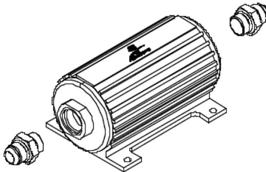
1-6. Noting the appropriate flow directions, install the provided AN-10 fuel filter, Aeromotive p/n 12301, on the fuel pump outlet and the AN-12 fuel filter, Aeromotive p/n 12302, on the fuel pump inlet.
