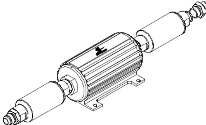
1-9. Find a suitable mounting location for the above pump / filter assembly. Typical mounting locations include mounting the fuel pump to the fuel tank shield or mounting to the inside of the frame rail. The fuel pump should be mounted as close to the fuel tank as possible and as low as possible. Using the fuel pump as a guide, mark the four pump mounting holes. Ensure there are no obstructions behind the mounting surface and drill four ¼" mounting holes.
