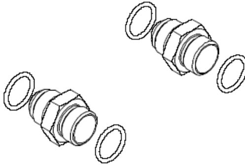
1-5. Install each of the two fittings into the appropriate end of the provided Aeromotive fuel pump.
