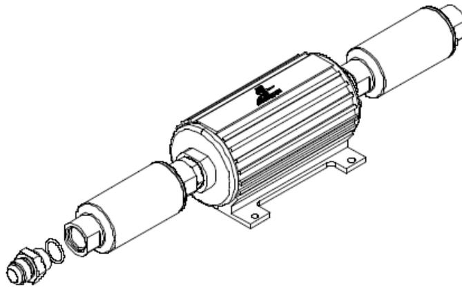
1-8. Install one of the supplied AN-10 o-rings on the AN-10 cutoff side of the AN-10 cutoff to AN-08 reducer union fitting, and install the fitting on the outlet side of the pump / filter assembly.
