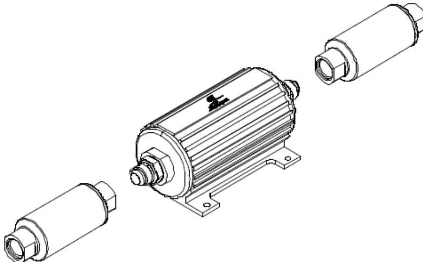
1-7. Install one of the supplied AN-12 o-rings on the cutoff side of the AN-12 cutoff to AN-10 reducer union fitting, if not already installed, and install on the inlet side of the pump / filter assembly.
