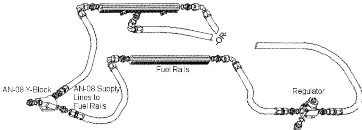
2-12. Starting from the outlet of the fuel pump / filter assembly, plan a route to run an AN-08 supply line from fuel pump / filter assembly to the Y-block, this line should be run along the same route you planned to run the return line in step 1.16. Cut the supply line to the determined length and install the AN-08 hose ends, as detailed in Section 3.
