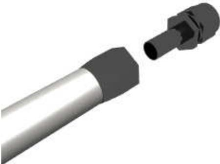
2-7. Using a properly sized wrench, complete threading the two components together (The maximum allowable gap between the two fitting components is .030 inches).
