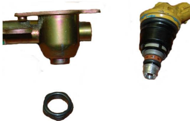
15. Remove the old o-rings from the fuel injectors, inspect the injectors for any dirt or debris and clean if needed. It is suggested that the old o-rings be replaced, contact your local auto parts store for replacement o-rings.
