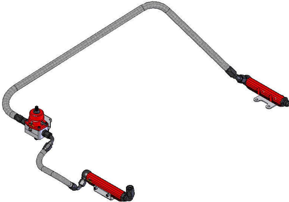
37. Install one ORB-06 o-ring on one of the AN-6 to 5/16 barb adapter fittings. Install the o-ringed side into the ORB-06 inlet port of the supply tee adapter fitting.
