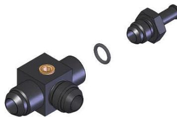
38. Connect the AN-08 straight hose end to the straight-through AN-08 male flare on the supply tee adapter. Plan a route for the line between the supply tee adapter and the AN-08 90-degree male ORB Hose end located in the front of the passenger (right) side fuel rail. Measure the length of fuel line needed and cut. See section titled Hose and Fitting Assembly for fuel line assembly instructions. Once the hoses are assembled, **ensure there is no debris in the hose** and install it.
