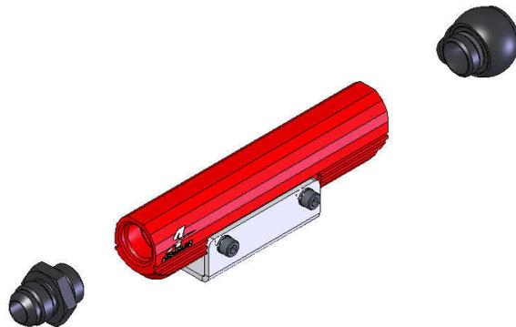
34. Reinstall the driver side “Fuel Pipe Protector” to insure that the rail and fittings have adequate clearance, the front edge of the “Fuel Pipe Protector” may need cleared to allow room for the hose end that threads onto the AN-08 union fitting on the front of the fuel rail.
