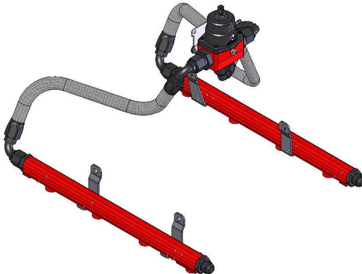
31. Inspect the OEM fuel supply line o-rings and replace if necessary. Place a light coat of oil on the fuel supply line o-rings and the supply line adapter fitting to ease installation. Connect the P/N 15102 OEM Spring Lock to AN-08 tee adapter fitting onto the OEM fuel supply line.
