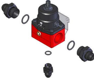
25. Install one AN-08 o-ring on the port (cut-off) side of each of the four P/N 15607 ORB-08/AN-08 port fittings.
