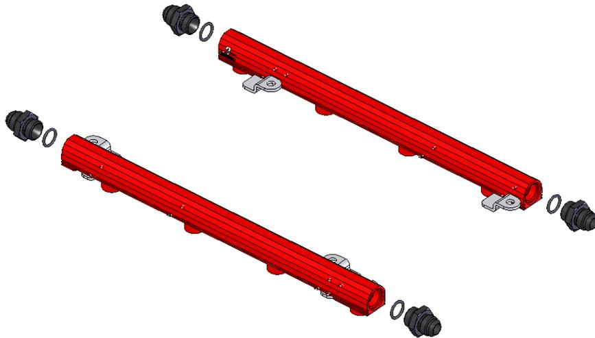
27. Inspect the OEM fuel supply line o-rings and replace if necessary. Place a light coat of oil on the fuel supply line o-rings and the supply line adapter fitting to ease installation. Connect the AN-08 tee adapter fitting p/n 15102 to the OEM fuel supply line.
