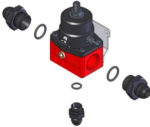
25. Install one ORB-08 o-ring on the port (cut-off) side of each of the four P/N 15607 ORB-08/AN-08 port fittings.
