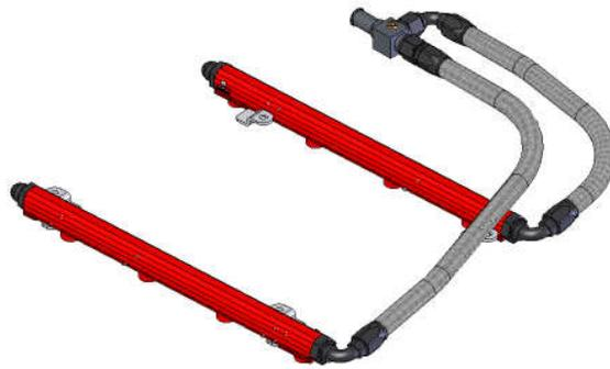
29. Connect one AN-08 90-Degree hose end to the rear of each fuel rail and one to each side port on the regulator. Plan a route for each of the two lines between the regulator and the fuel rails. Measure the two lengths of fuel line needed and cut the line. See section titled Hose and Fitting Assembly for fuel line assembly instructions. Once the hoses are assembled, **ensure there is no debris in the hose** and install them.
