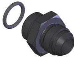
19. Thread the o-ring side of the 15607 AN-08 fitting, into each of the two ORB-08 ports on ends of the fuel pressure sensor adapter.
