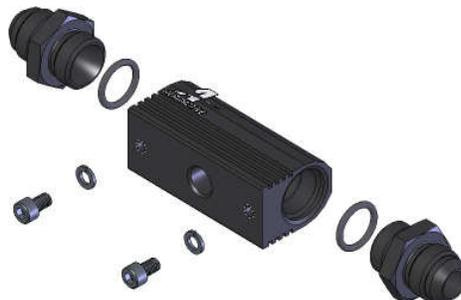
19. Thread the o-ring side of each P/N 15607 port fitting into the front and back ports of each fuel rail.
