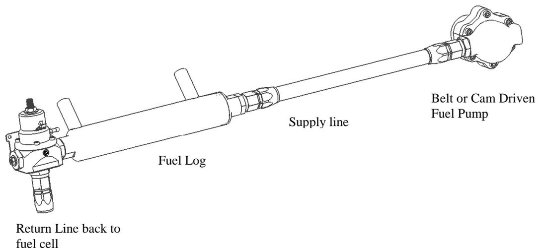
5. Attach the fuel log supply line to the AN-10 port located on the side of the regulator using AN-10 style fittings and o-rings.
