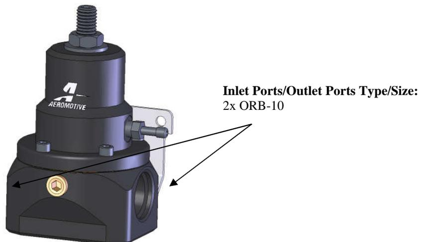
7. Attach the fuel return line to the ORB-10 bypass port located at the bottom of the regulator using a ORB-10 to AN-10 port fitting (Aeromotive P/N 15608 or equivalent) and o-ring.
