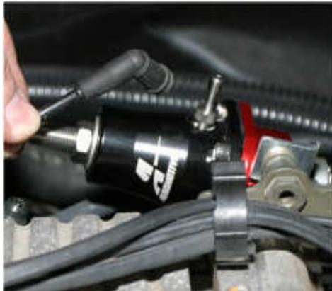
12. Once the regulator is installed, attach a suitable fuel pressure gauge to either the fuel system schrader valve or the 1/8-NPT gauge port.
