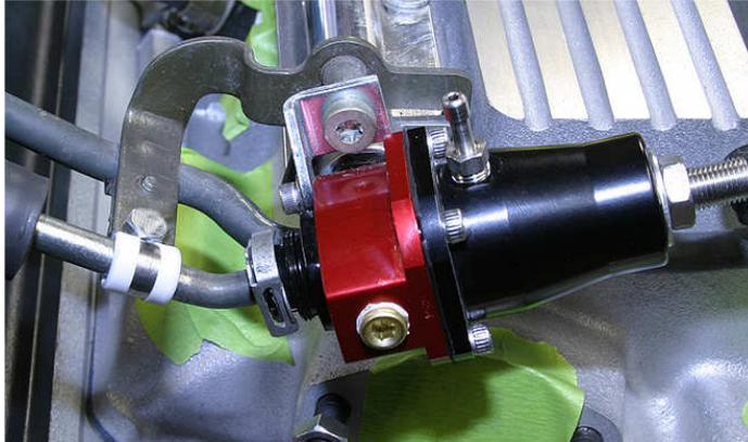
11. It also may be necessary to extend the OEM vacuum/ boost reference line using the enclosed barb union and section of vacuum hose to achieve the desired line routing.
