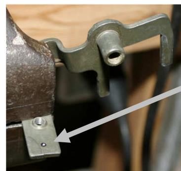
10. Using the enclosed self-threading screw and cushioned line clamp mount the OEM return line in its new location
