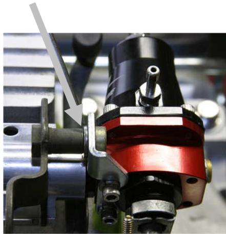
9. In some installations it may be necessary to relocate the return line mounting clamp. Using the enclosed cushioned line clamp as a pattern, mark the OEM line bracket and drill a hole using a #18 drill bit (.170 Diameter).
