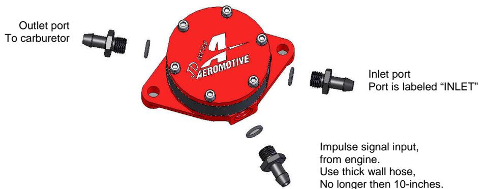
7. Connect the 5/16" barb fuel pump outlet to the carburetor fuel supply line.
