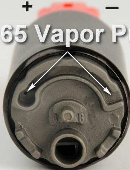
**Warning:** Note the location of the vapor-purge port / channel openings at the bottom of your new 325 Stealth Fuel Pump, as illustrated above. Be certain to check for and eliminate any restrictions to this port during installation. Failure to do so may cause slow or no priming, resulting in difficulty starting the engine and permanent damage to the fuel pump.
