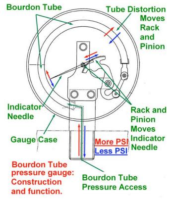
The mechanism used in a typical mechanical pressure gauge is ingenious, and of course depends on basic physics to work correctly. When installed, fuel system pressure is directed into the Bourdon Tube, inside the gauge, through the test port. Changes in fuel pressure are then applied to the inside of the Bourdon Tube, causing it to change shape or distort.
